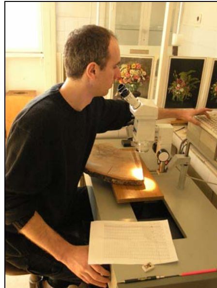
Measuring ring widths from Fagus sylvatica disks at the laboratory
